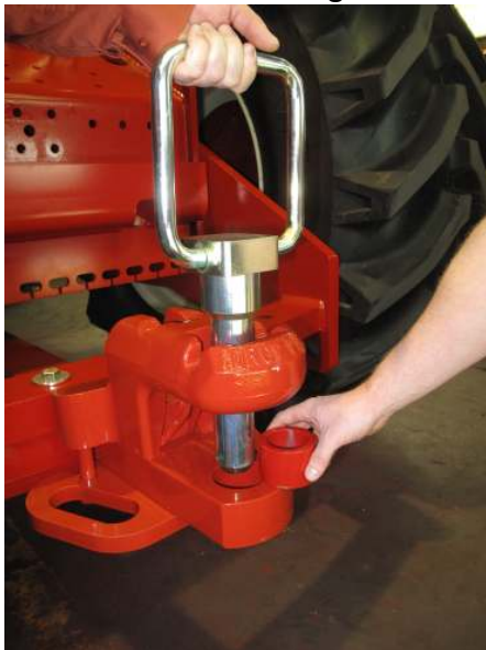
The adapter bushing drops into the drawbar.
